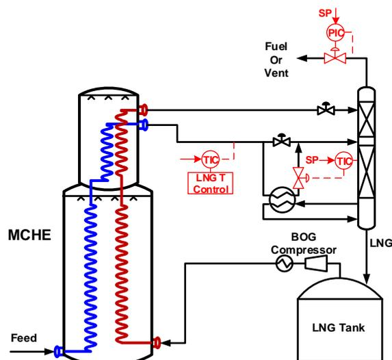
Figure 6. Nitrogen Removal Scheme with Dedicated Circuit for Recycled BOG (Patent Pending)
