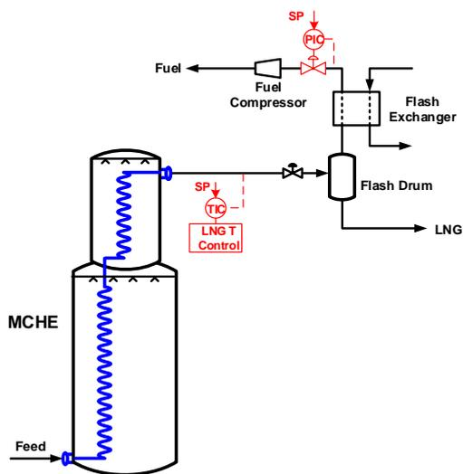
Figure 2. LNG end flash drum
