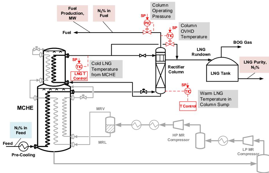
Figure 7. Simplified PFD used in the Dynamic Simulation
