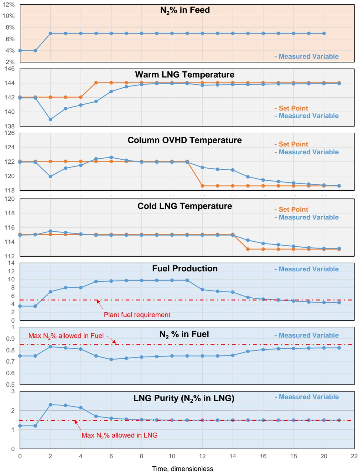
Figure 8. Dynamic behavior of the system with increased nitrogen content in feed gas
