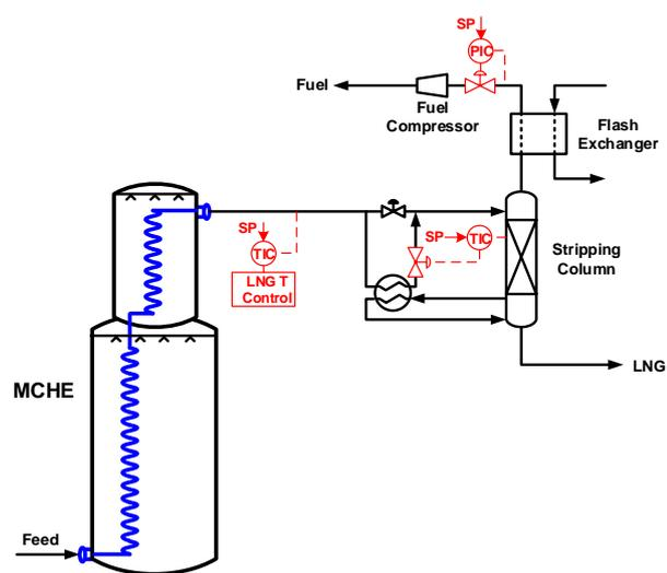
Figure 3. Nitrogen Stripping Column
