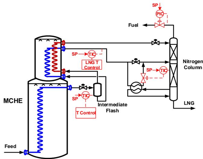
Figure 5. Nitrogen Removal Scheme with Dedicated Circuit for Intermediate Flash (Patent Pending)
