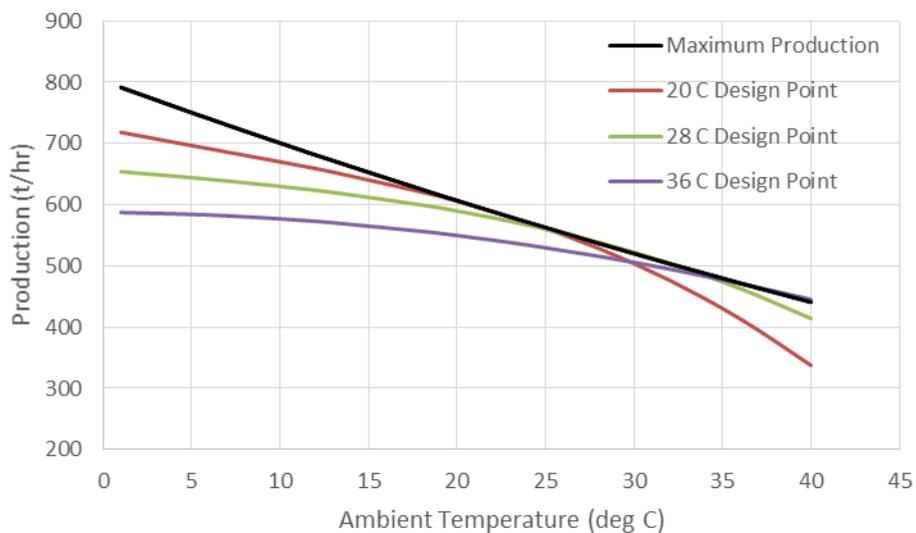
**Figure 2. LNG Production over a Range of Ambient Temperatures.**
