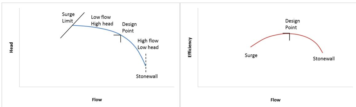
**Figure 3. Effect of Flow on Compressor Operation.**
