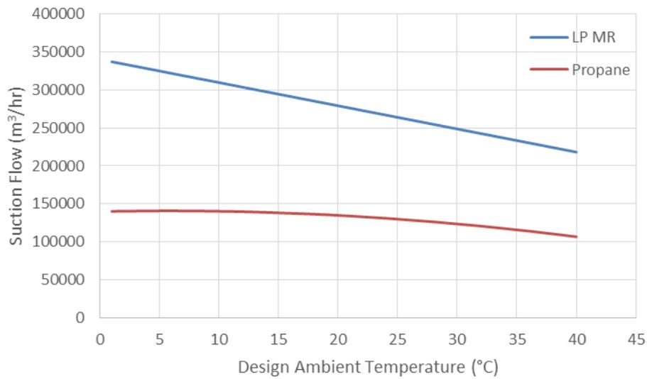
**Figure 1. Design Case Compressor Suction Flow.**
