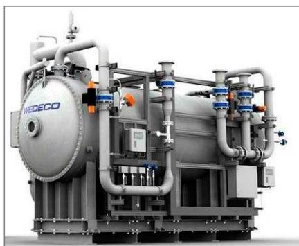
Pictured above is a large scale ozone generator which generates ozone at 6 to 15 wt% from an oxygen feed gas. The generated ozone stream is directed to the O<sub>2</sub>/O<sub>3</sub> SLR process for separation of oxygen and creation of an ozone containing nitrogen gas.
