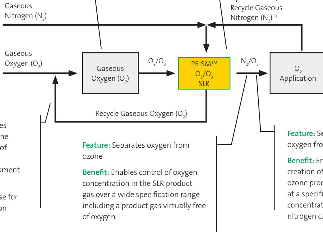
**Feature:** Separates oxygen from ozone enabling recycle of oxygen to ozone generation equipment
