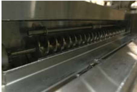
Foam-insulated cooling conveyor – ideal for applications that require frequent material changes
