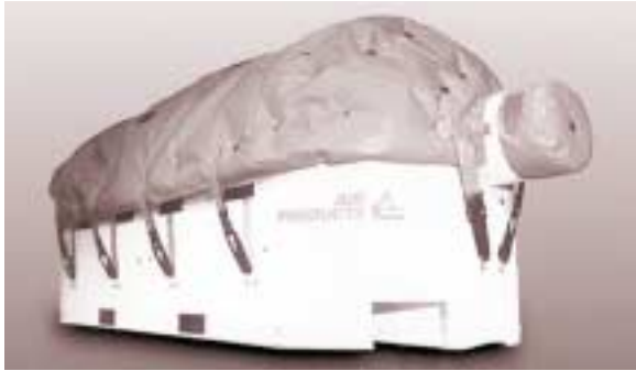
Figure 3. A BSGS fitted with a bulk container heater.
