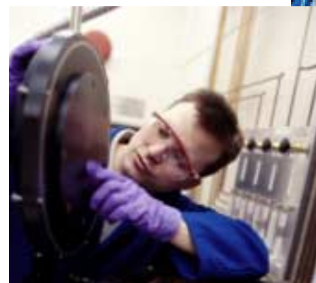
Inspecting the etching reactor in Air Products' Semiconductor Processing Applications Research Laboratory at Allentown. As a result of facility and equipment upgrades, a commercial-scale cluster tool, capable of processing eight-inch wafers, is now being employed to support a variety of research and customer support projects.
