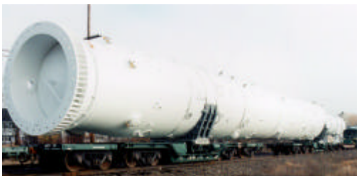
Fig. 3 Coil wound MCR® cryogenic heat exchanger ready for shipment on side shifting rail car.
