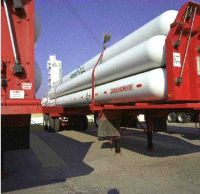
Typical Carbon Monoxide Tube Trailer
