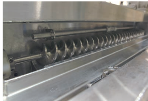
Foam-insulated cooling conveyor
