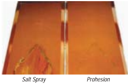
Figure 3: Epilink® 701 Metal Primer (ACP01) Panels Following 1000hrs Accelerated Weather Tests
