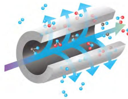
**Note:** the PB6050-P3 membrane system was originally designed with a vacuum sweep to remove the hydrogen that permeated into the separator shell, but the flow design efficiency eliminated the need for vacuum pumps to meet the target hydrogen concentrations.
