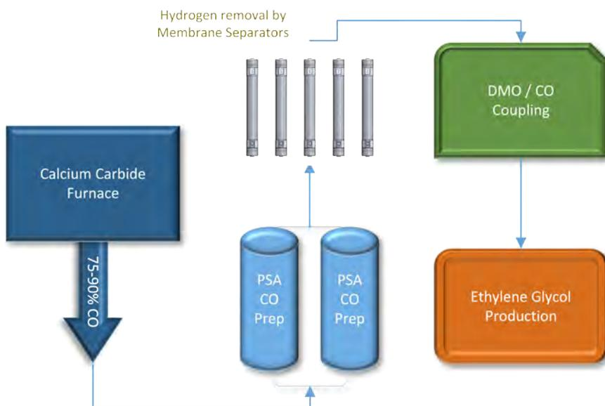
The process begins with the generation of carbon monoxide in the tail gas of a calcium carbide furnace. The tail gas contains 75–90% carbon monoxide with hydrogen molecules and other impurities. Typically, these systems use a palladium catalyst reaction to remove hydrogen from the tail gas stream. In the presence of a catalyst (palladium which is very expensive) the hydrogen ions will be removed but there are secondary reactions that cause a buildup of carbon
