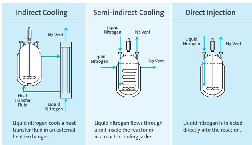
Careful selection of the cooling system is critical in establishing a robust and safe manufacturing process:
