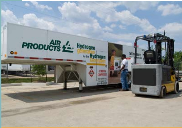
Air Products mobile Hydrogen Fueler provides hydrogen fuel for a customer's forklift.
