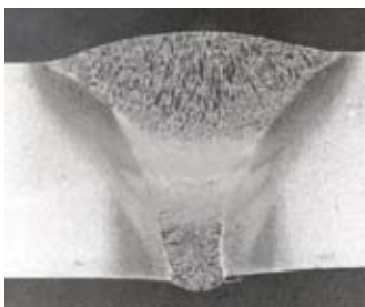
PA MAG (135) single sided butt weld in 3mm thick carbon steel using Ferrolinx U.
