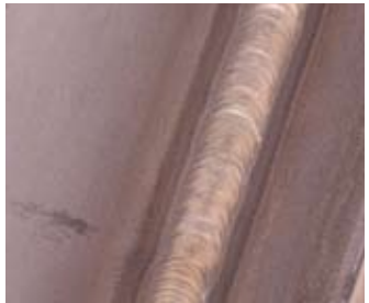
PB TIG (135) fillet in 3mm austenitic stainless steel using Inolinx TIG.
