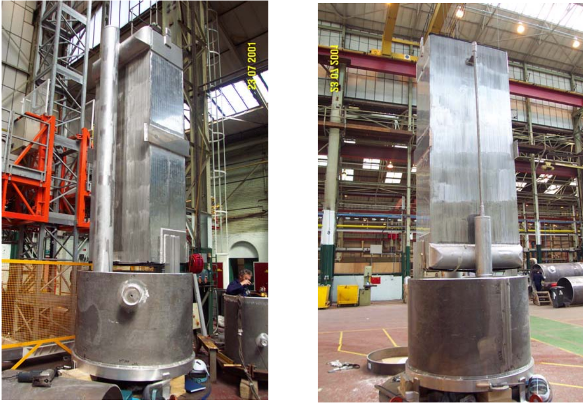
Figure 5 Reboilers in Construction
