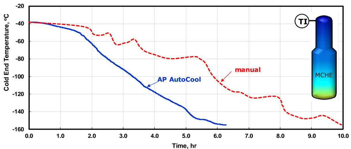
Figure 4: Automated vs Manual Cooldown
