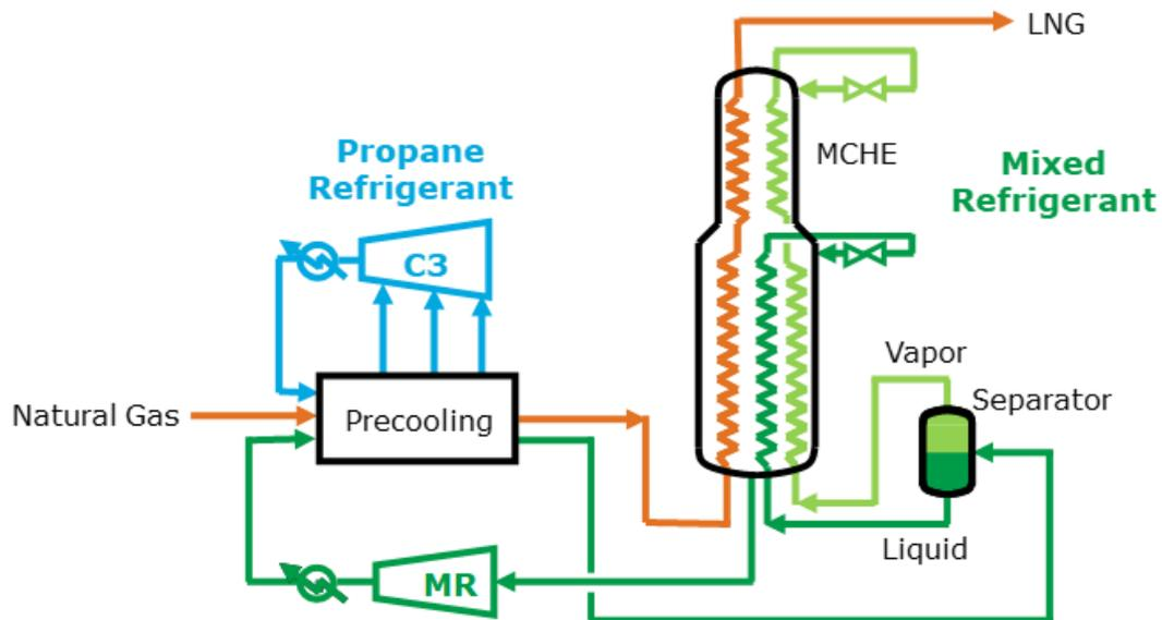
Figure 1: Air Products' AP-C3MR LNG Process
