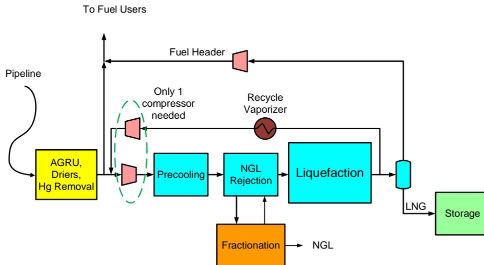
Figure 6: Reduced Flaring LNG Block Diagram
