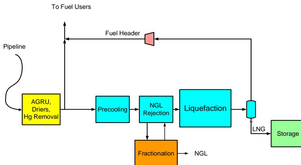
Figure 5: Typical LNG Plant Block Diagram
