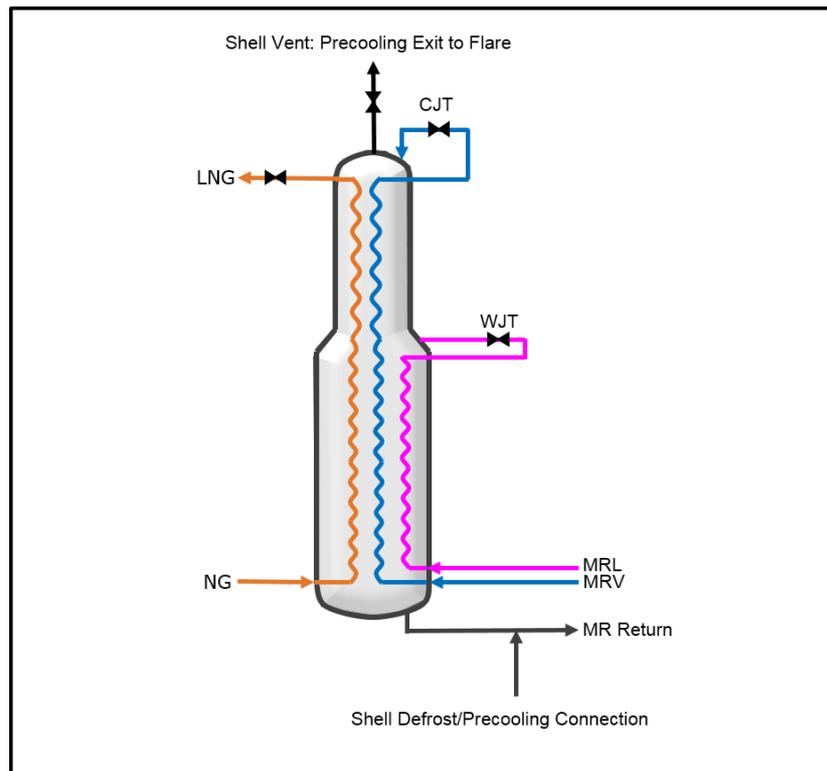
Figure 2: Precooling Flow Path
