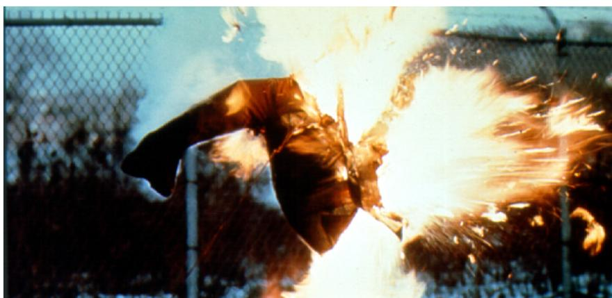
Figure 2 shows a normal cotton work shirt, stuffed with paper and saturated with oxygen. Inside the shirt is a simple ignition device. The results of the ignition are shown in Figure 3. Individuals must be aware of the hazards of oxygen enrichment, since oxygen is not detectable by human senses. It is colorless, odorless, tasteless and nonirritating. Likewise, they must be aware where oxygen enrich-
