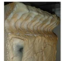
Accelerated refractory wear at metal line due to corrosive nature of foam
