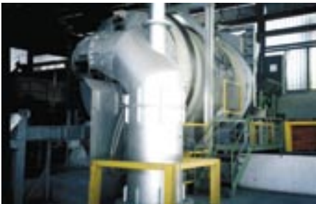
Figure 3: A fixed-axis rotary furnace using APMELT™ LEAM® technology and equipment
