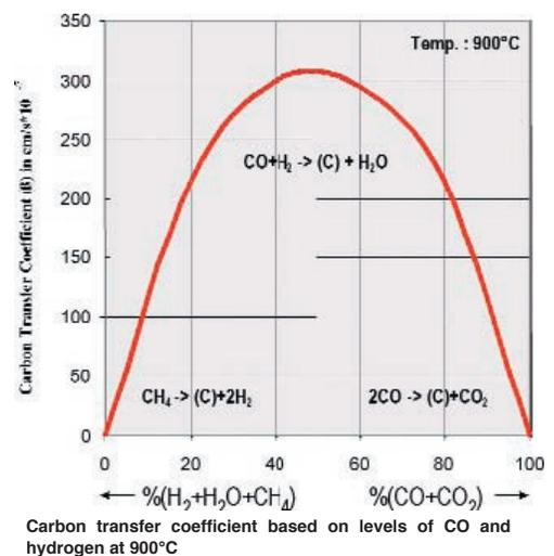
**Guido Plicht and colleagues from Air Products report on the development and implementation of a new mass flow controller system that measures the carbon monoxide (CO) level in a furnace during the carburisation process and thereby allows greater reliability and uniformity of the treatment process, speeding up productivity – as demonstrated during recent trials with Mubea in Germany**
