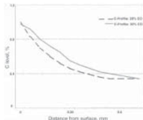
4 Carbon profile of carburised steel with 20%CO compared with carburised steel with 30%CO and 15% less carburising time
