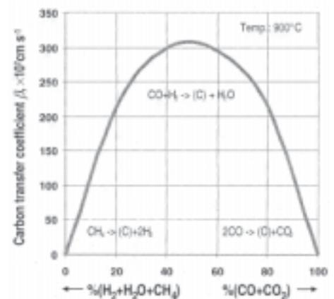
1 Carbon transfer coefficient based on CO and H<sub>2</sub> levels at 900° C: after Ref. 3
