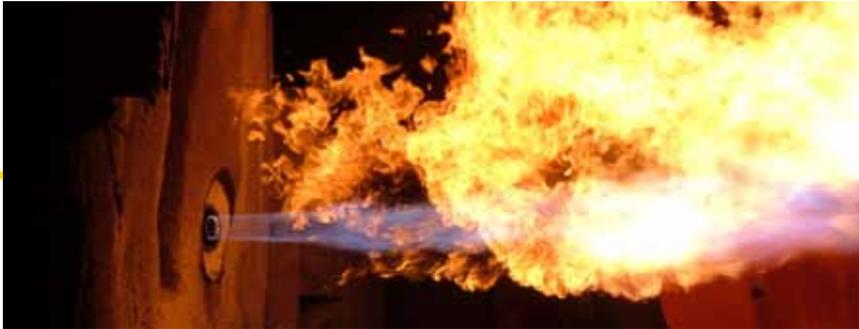
Air Products' patent pending\* burner technology minimizes melt losses and flux usage while achieving improved productivity, reduced process costs and emissions. The Air Products High-Yield Oxy-fuel Burner was designed specifically to increase yield for secondary aluminum melters. Our combustion researchers used state-of-the-art computer modeling – with extensive operational data from melting operations – to develop a new generation burner.
