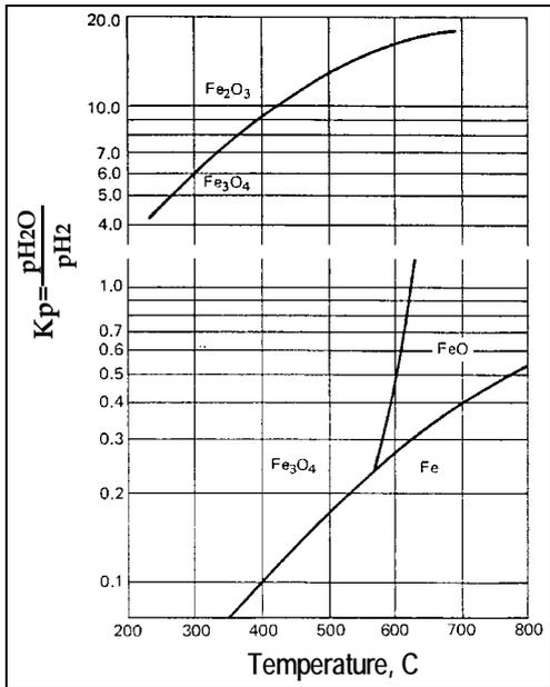
Figure 1b. Equilibrium Phase Diagram (Kp vs. Temperature) for Alloying Elements
