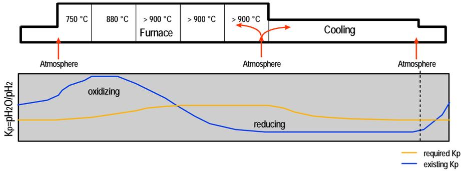
Figure 3. Schematic of the Advanced Atmosphere Monitoring and Control System
