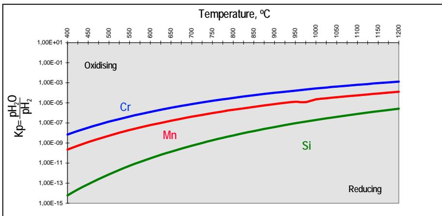
Figure 2. Reducing and Oxidizing Potential of Atmosphere Present Inside a Continuous Furnace
