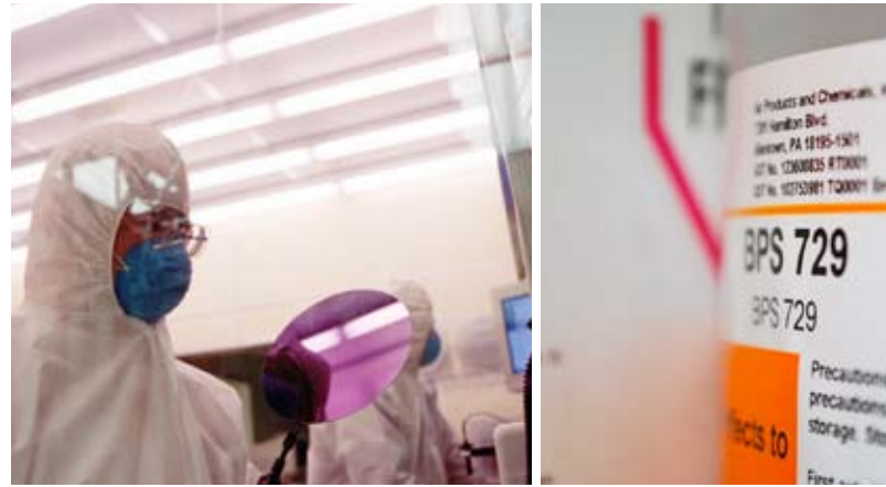
Air Products' Better Process Solutions (BPS) wet chemistries are an efficient and simple way of removing metal oxides, fluorine, particulate contamination, organic residues, and flux from wafers with out damaging the underlying metals.
