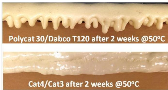
**Figure 12.** Machine sprayed samples, foam edge after three passes to show foam dripping and lack of cure.
