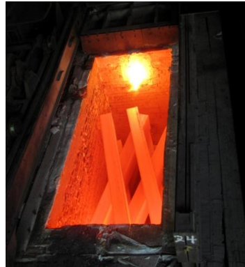
Figure 2: Photograph of a soaking pit furnace at ArcelorMittal's facility in Steelton, Pennsylvania
