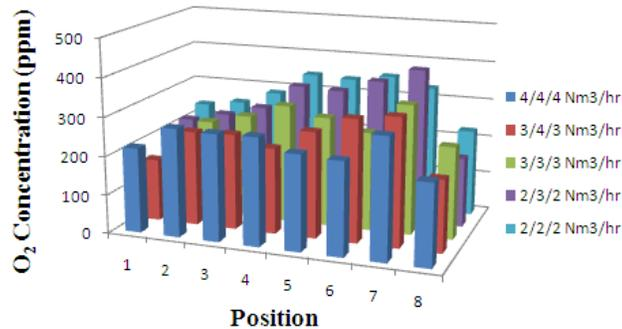
**Figure 11: O<sub>2</sub> Distribution around Solder Pot**
