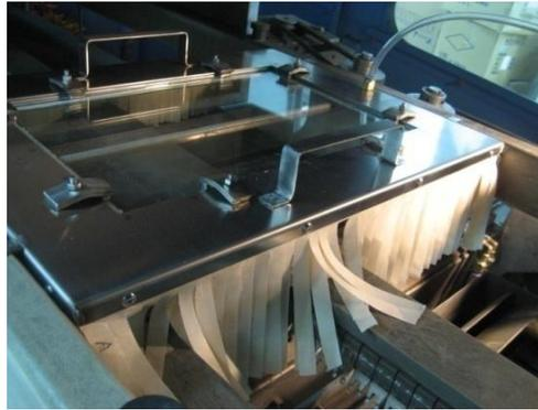
**Figure 18: Top Cover with Flexible Curtains on both Sides**
