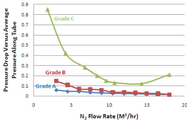
**Figure 2: Permeability Test Result for Selecting Diffuser**
