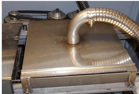
**Figure 16: Collecting Flux Vapor using the Top Cover**
