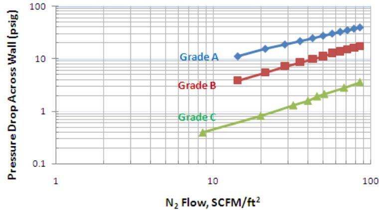
**Figure 3: Permeability Test Result for Estimating Flow Resistance** Figures 4 and 5 are two examples of the modeling results. One is O<sub>2</sub> distribution across a solder pot with dual waves and the other is a side view of N<sub>2</sub> flow field for a specific design under a given process condition.
