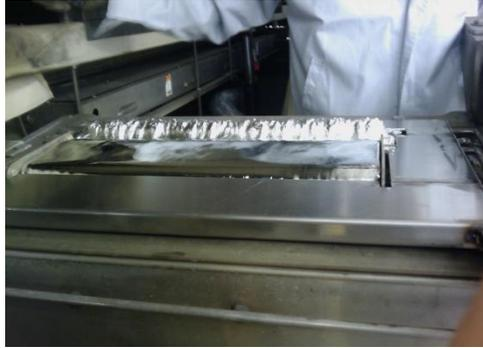
**Figure 17: Protective Housing Inserted in a Solder Pot with Two Waves**
