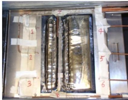
**Figure 13: Solder-Free Middle Diffuser**
