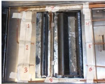
**Figure 10: Eight Sampling Tubes Around Solder Pot**
