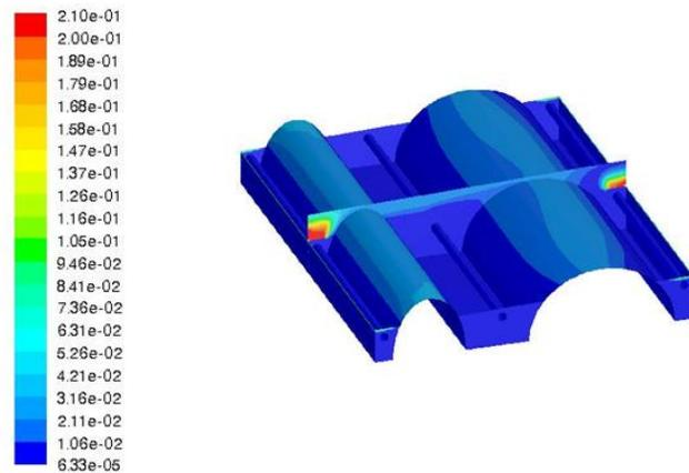
**Figure 4: An Example of 3D Modeling Result on O<sub>2</sub> Distribution**
