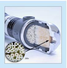
A typical membrane separator contains thousands of fibers that are bundled and encased at both ends in epoxy resin. The ends of the bundles are cut, which leaves the fiber bores open on both ends, allowing the gas to travel from one end to the other. The bundles of fibers are enclosed in a suitable casing. The casing protects the fibers and routes the gas properly.
