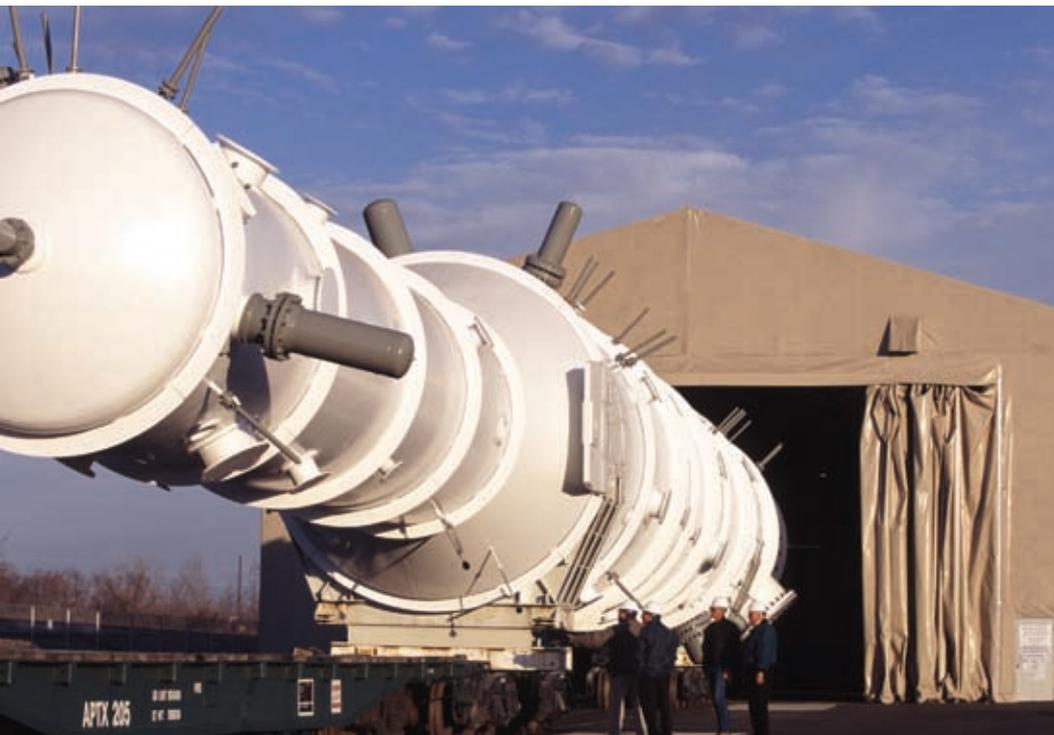
*MCR main cryogenic heat exchanger during manufacture.*
