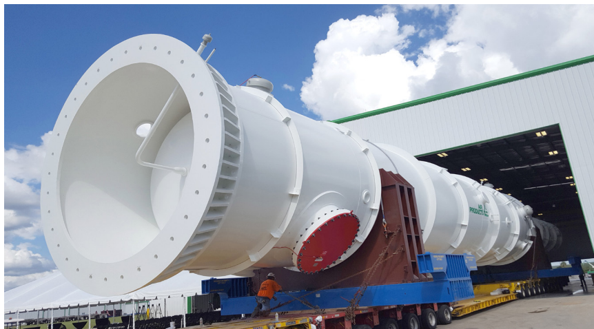
A large Air Products' custom designed coil wound heat exchanger.
