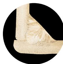
Inomaxx® 2 MIG fillet weld in 3mm thick AISI 316L stainless steel
