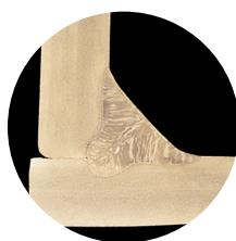
Inomaxx® Plus MIG fillet weld in 6mm thick AISI 316L stainless steel
