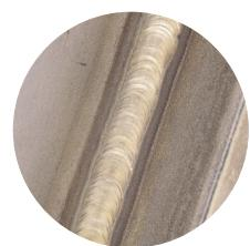
Inomaxx® TIG butt weld in 3mm thick AISI 316L stainless steel
