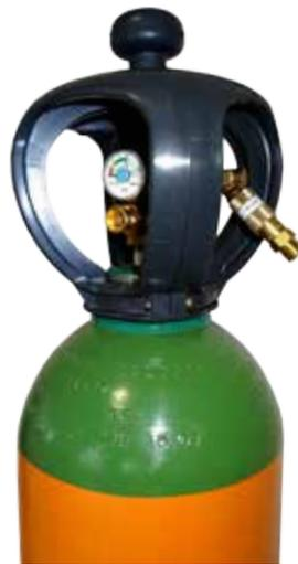
Specially designed for the Air Products 200 bar Integra cylinders. No need for extra regulators, as the outlet pressure (4 bar) and flow are preset. Simply change the optimizer and with one click you have the correct gas flow. The flow optimizers are available with a flow of 8, 10, 12, 15, 18, 20 and 25 L/min.
