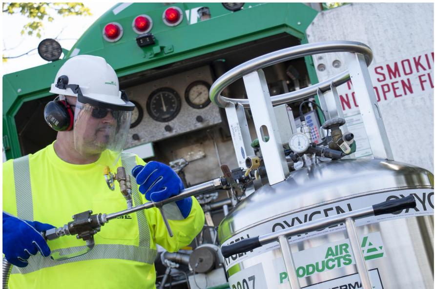
The Osceola facility also provides CryoEase® Microbulk Solutions, a cost-effective alternative for small volume supply that fills on-site vs. the traditional method of swapping empty for full cylinders and dewars.
