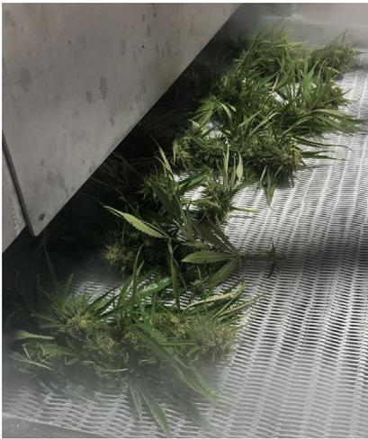
Freezing industrial hemp using a cryogenic liquid-nitrogen system can offer a cost-effective, faster alternative to traditional methods of drying and storing. Plus flash freezing retains more of the valuable cannabinoid compounds in the hemp product.
