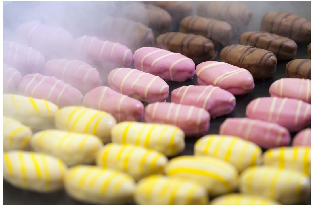
Cooling food surfaces with nitrogen can help alleviate issues with taffy cooling, product layering, die jamming, fixture handling or sticking, and much more. When a decorative drizzle turns into a puddle or a seven layer cake looks like three, targeting very cold nitrogen gas at the problem area might be the solution.
