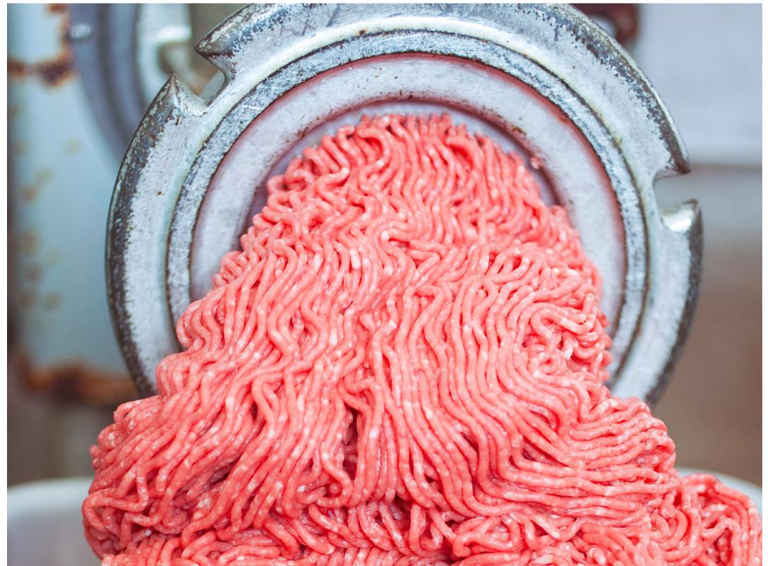
Liquid nitrogen can be used to help maintain the cold temperature of the meat through a controlled injection directly into the product during mixing/grinding. The nitrogen injection is regulated to provide the cold that is required at all times, adjusting the liquid nitrogen consumption to the requirements of the process.
