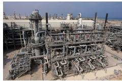
The company strengthens its worldwide leadership in natural gas liquefaction process technology by introducing a debottlenecking process that enables as much as a 60 percent capacity increase in production without sacrificing existing efficiency. **Pictured:** A main cryogenic heat exchanger, which is part of Air Products' AP-X® liquefaction process technology.
