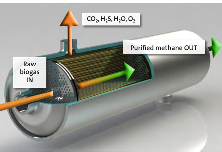
**PRISM membrane separators for biogas upgrading contain thousands of tiny hollow fibers. Smaller gas molecules, like carbon dioxide and water vapor, diffuse through the membrane walls while the larger methane molecules are transported the length of the tube and exit from the end of the module.**
