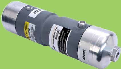
Air Products' CACTUS PC dryers are compact and efficient dehydrators for industrial air supplies. These robust dryers remove water vapor from gas streams by the selective permeation of water molecules through polymers. They are “molecular filters” in which water travels across the membrane faster than other gas molecules.
