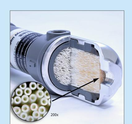
A typical membrane separator contains thousands of fibers that are bundled and encased at both ends in epoxy resin. The bundle ends are cut, which leaves the fiber bores open on both ends, allowing the gas to travel from one end to the other. The fiber bundle is enclosed in a suitable casing. The casing protects the fibers and routes the gas properly.
