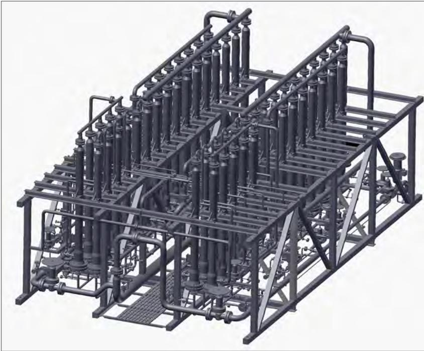
Typical oil refinery systems produce hydrogen with purities between 90 to 98 mol%. Product gas purity is dependent upon feed composition, available differential partial pressure and required hydrogen recovery level. The hydrocarbon-rich stream is returned at nearly the same pressure as the feed gas for use as fuel gas.
