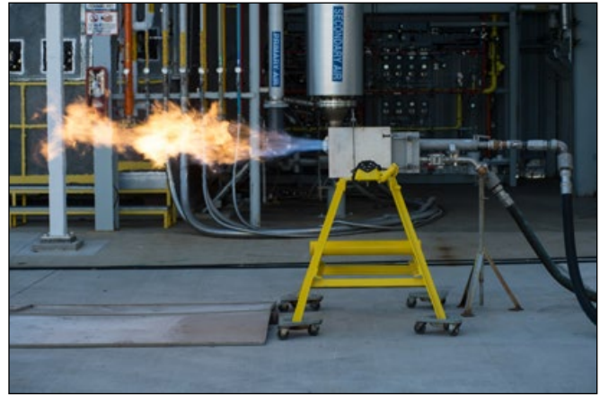
Figure 3. Adjustable heat release oxy-fuel burner.
