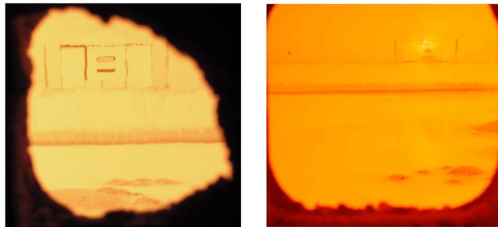
Operation of the HR<sub>x</sub> burner in the Foam Control mode (right) generates a reducing environment adjacent to the glass surface that destabilizes surface foam (left), yielding higher flame-to-glass heat transfer rates and improved glass refining.
