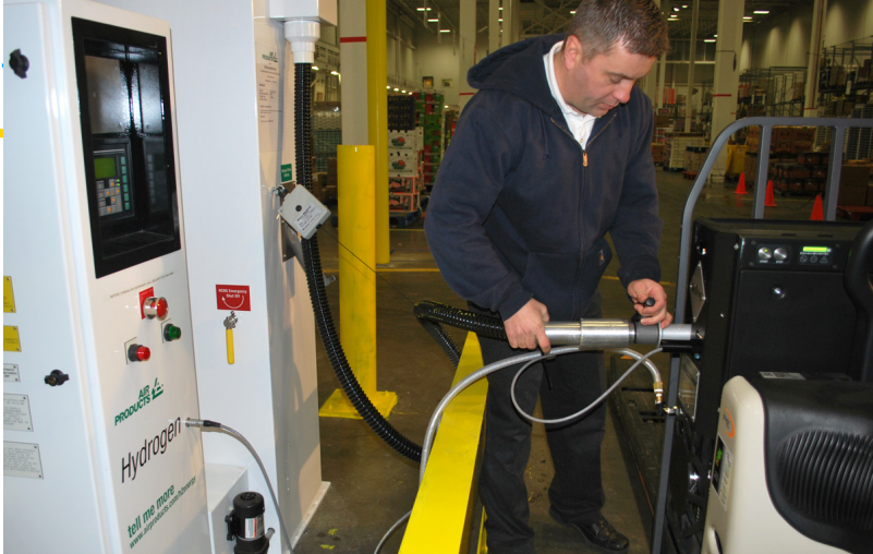
Air Products' hydrogen fueling system provides hydrogen fuel for a customer's forklift.
