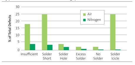
Inert Gas Wave Soldering – dross reduction versus atmosphere purity
